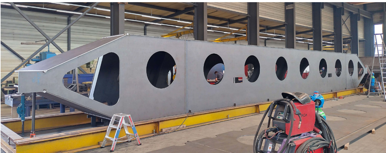
The new welded stop logs
