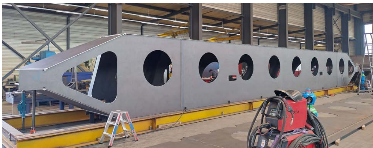
The new welded stop logs
