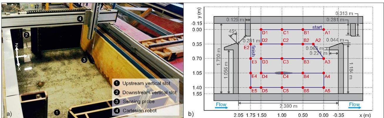
Figure 3. Experimental setup of the KIT fish pass. Right: locations and orientation of the investigated basin. Left: schematic showing the dimensions as well as the horizontal (x,y) measurement locations taken for a single vertical position of the probe.
