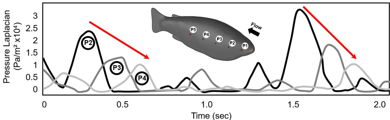
Figure 4. Two vortex events recorded using the LLP pressure Laplacian. The red arrows show the cascade of the Laplacian as the vortex core passes along right lateral sensors P2, P3 and P4. The negative slope indicates that the vortex strength is decreasing over time.
