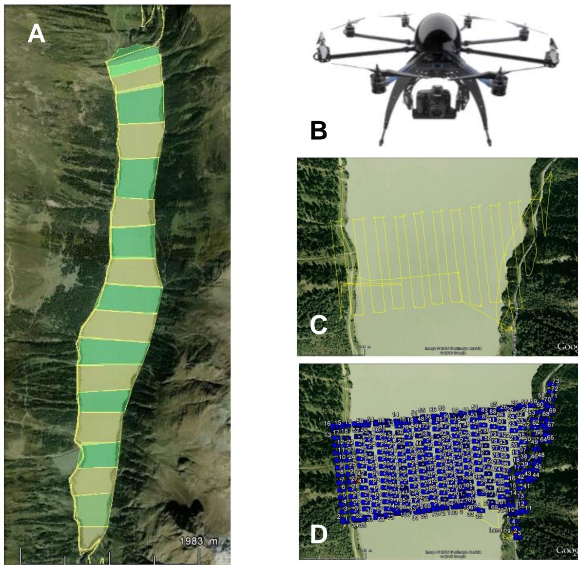
Figure 1. Gepatsch reservoir, A – overview on the 20 flight sectors (uppermost = 20), B – UAV MULTIROTOR service-drone, C – example for flight planning in sector 8 and D – corresponding camera positions
