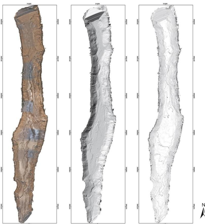
Figure 2. Orthophoto and DEM of the Gepatsch reservoir (December 2015)
