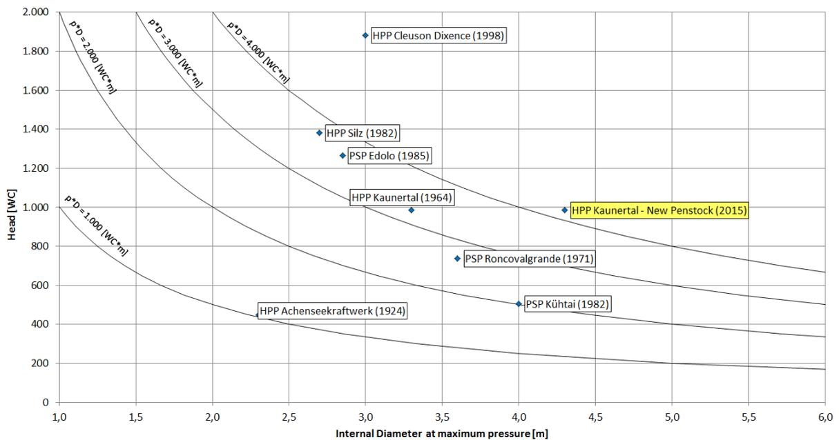
Figure 2: Criticality of penstocks due to pressure and size
