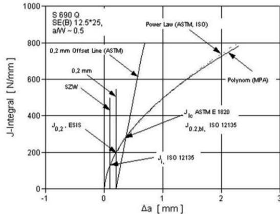
Figure 6: Different crack initiation and resistance values [6]
