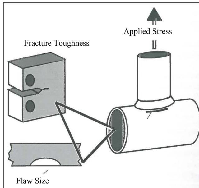
Figure 5: Fracture mechanics triangle [7]
