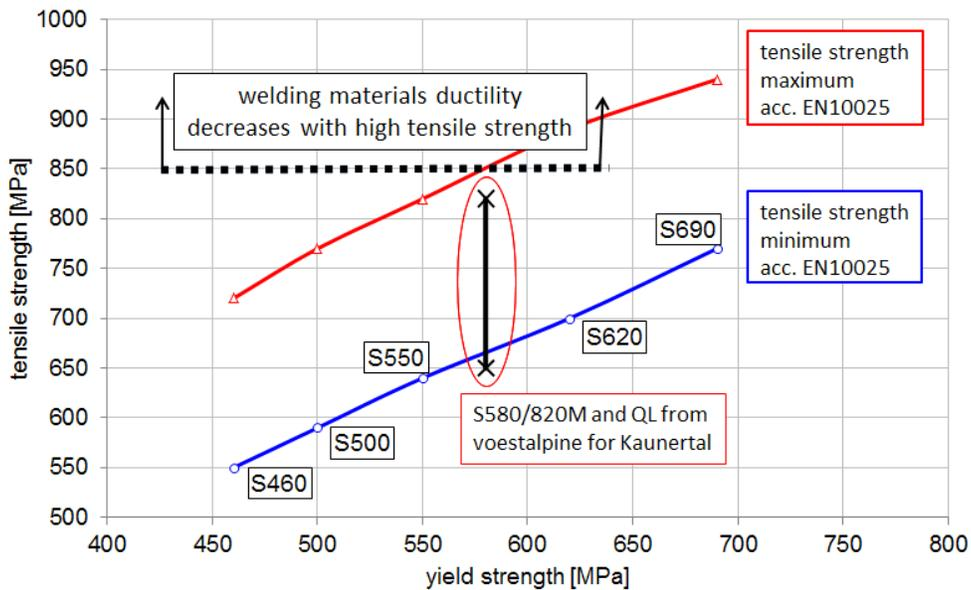
Figure 4: Standard specification of strength according to EN10025[6]
