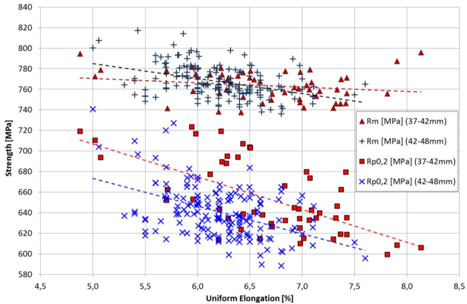
Figure 3: Relation of Strength and Uniform Elongation on TM-Steel Alform580/820 for the Kaurertal penstock
