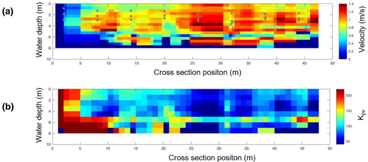
Figure 4. (a) ADCP 50 cm raster of the flow velocity in front of the Kirchbichl hydropower intake at 250 m<sup>3</sup>/s, positions of the pitot measurements are shown in grey. (b) Map of the turbulence parameter  $K_{pv}$  based on the regression model fit from the measured locations.
