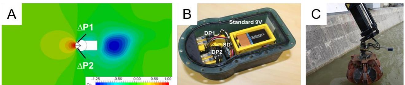
Figure 2. (A) CFD results showing the locations of the differential ports and distribution of the pressure coefficient,  $C_p$  for a freestream velocity of  $10 \text{ cm/s}$ . (B) Photograph of the device including the two differential pressure sensors, DP1 and DP2 as well as the power supply and data storage card. (C) Image of the prototype in the field at the HPP Kirchbichl, mounted on the large debris removal arm.
