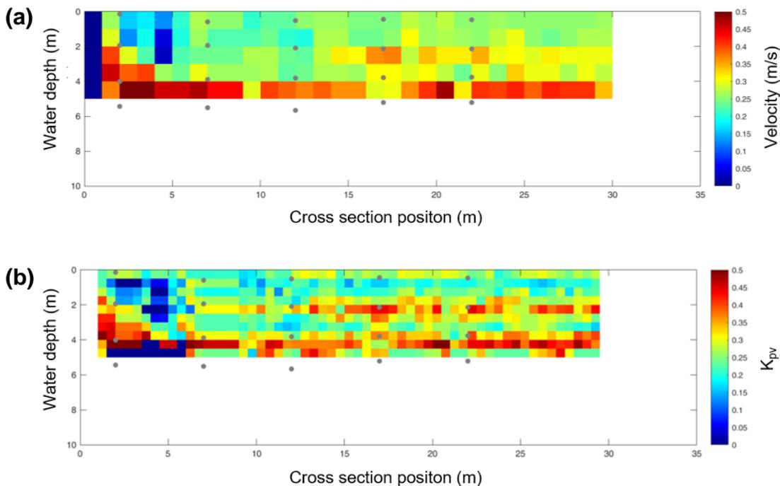
Figure 5. (a) ADCP 50 cm raster of the flow velocity in front of the Runserau intake at 30 m<sup>3</sup>/s, positions of the pitot measurements are shown in grey. (b) Map of the turbulence parameter  $K_{pv}$  based on the regression model fit from the measured locations.
