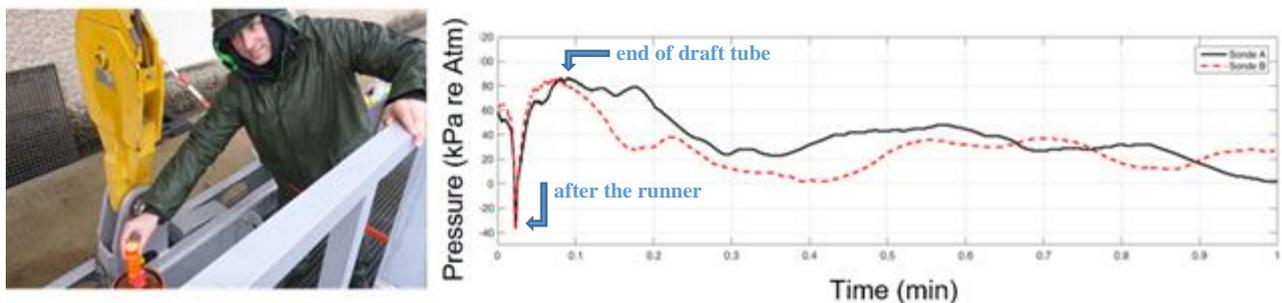
Figure 6. Left: Prototype BDS sensor being inserted into the hydropower intake. Right: Pressure time series recorded with two sensors (Sonde A and B), the sharp jump in the pressure readings for both sensors correspond to the passage through the turbine.
