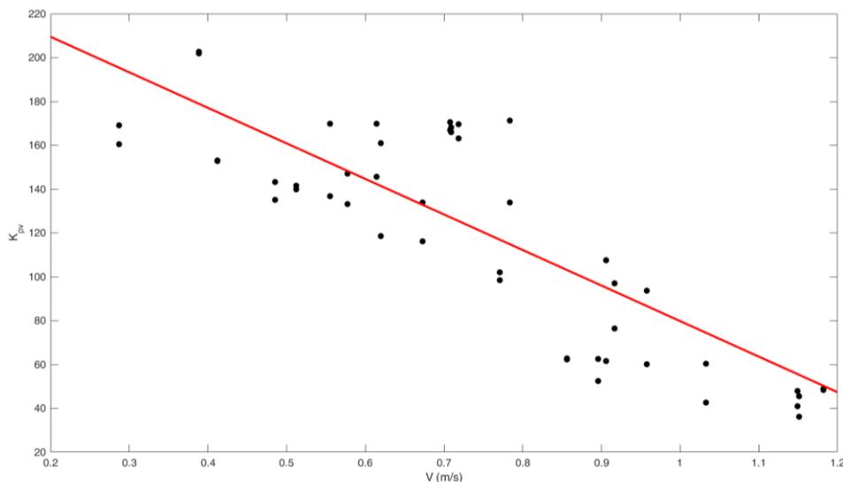
Figure 3. Correlation plot between the time-averaged velocity as measured by the ADCP and the corresponding  $K_{pv}$ , based on the measurements from HPP Kirchbichl (18.04.2016). The fit was made using linear least-squares regression ( $K_{pv} = -162,1 * V + 241,9$  ( $n = 48$ ,  $R^2 = 0,73$ )).
