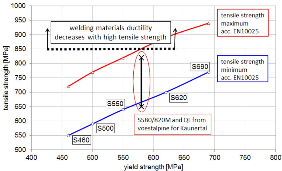
Fig. 1 Standard specification of strength according to EN10025
