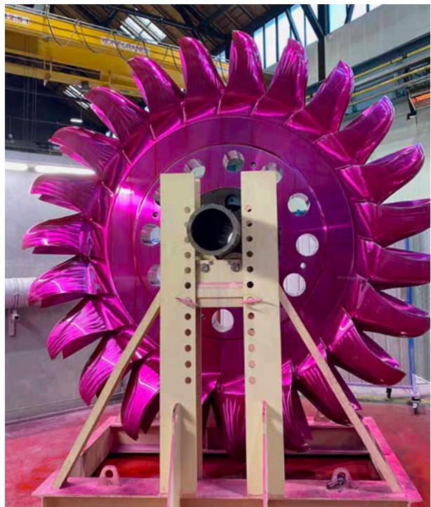
The new runner at so-called penetrant testing
